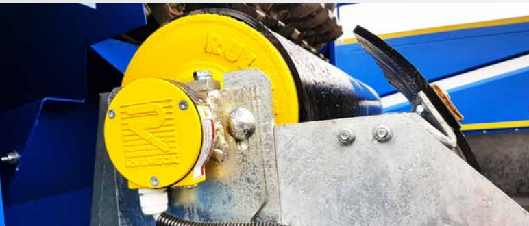
Electric conveyor belt drive
