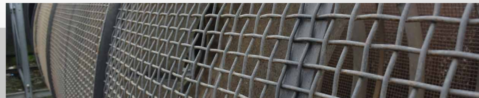
Screening trommel with wire segments
