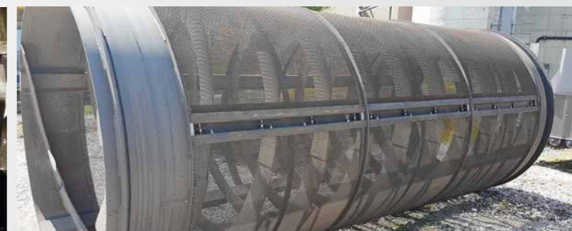
Screening trommel with wire segments
