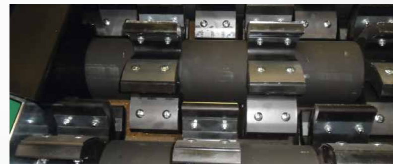
Wear plates on polyurethane screening stars
