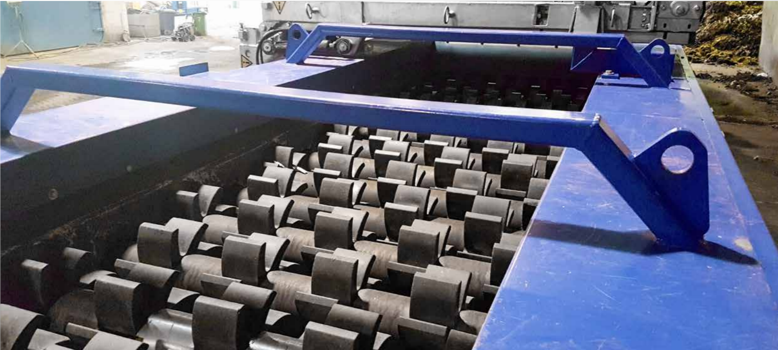
Cassette construction of the screening decks
