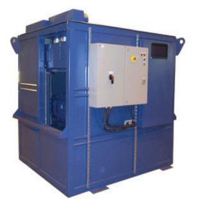
The PES 7 unit shall always be connected to a filter separator to complete a vacuum system
