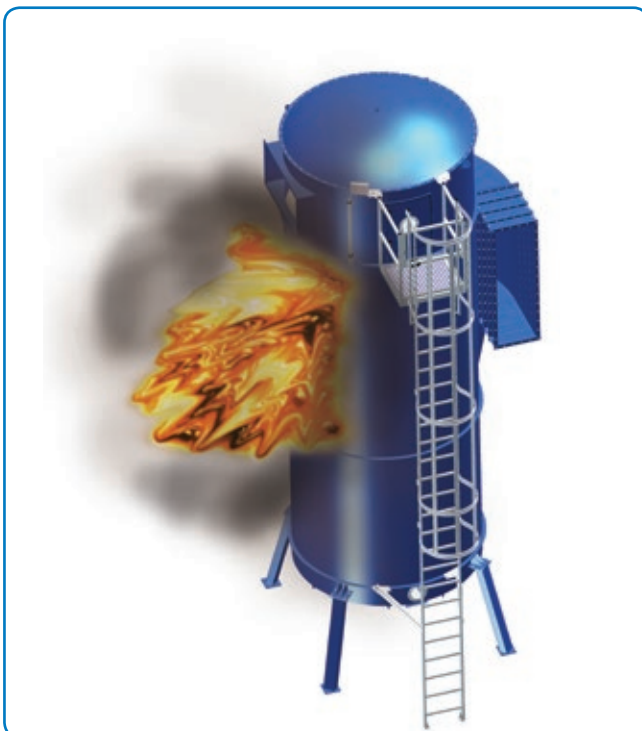
1. Explosion relief venting in the filter body
