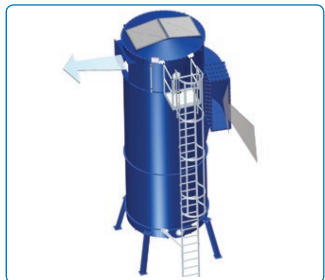
BF-filter with scraper bottom and tangential inlet. Shown with VFV® explosion relief venting in the filter top. Fitted with ladder and platform.
