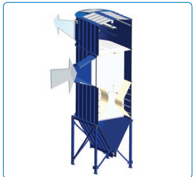
SBF filter with conical bottom and side inlet. Cross-section shows Coanda plates, used to accelerate and compress particles so that they settle to the bottom.
